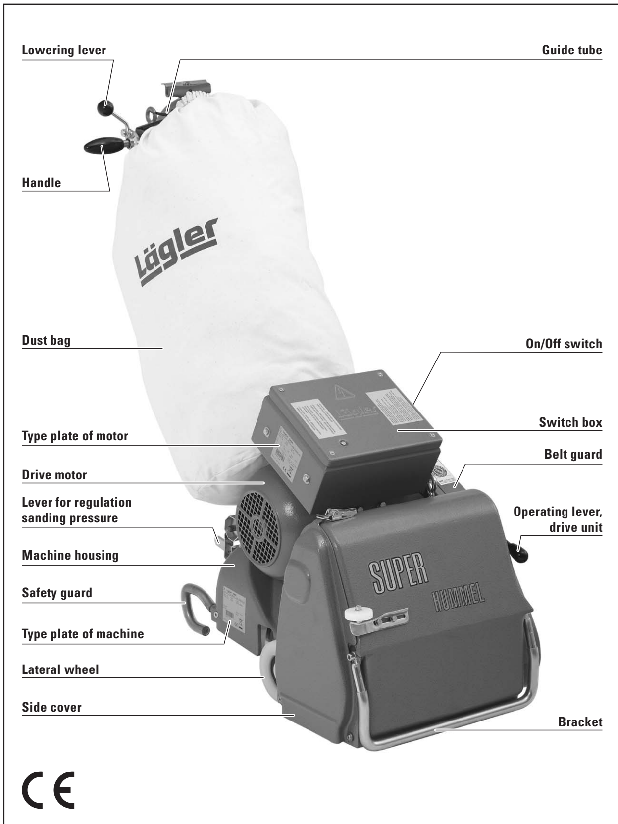
Fig. 1 Important parts and assemblies of the belt sanding machine SUPERHUMMEL
