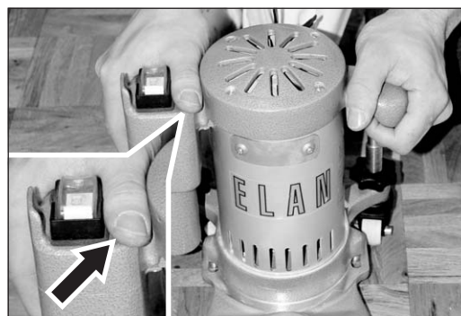
Fig. 13 Guide the ELAN with both hands. Do not touch the switch button while sanding!
