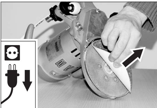
Fig. 21 After removing the sanding disc pull off the Velcro negative and clean the sanding plate.
