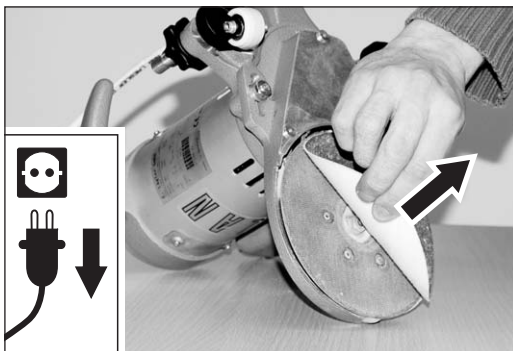
Fig. 16 Simply pull off the Velcro sanding disc.
