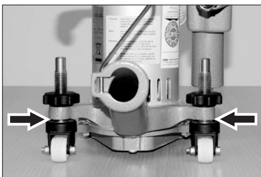
Fig. 57 Flat machine setting for fine sanding tasks.
