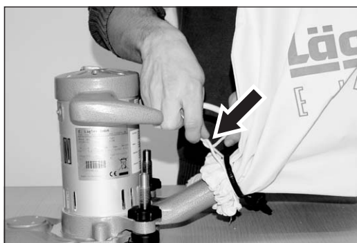
Fig. 7 Tying up the dust bag with the cord.
