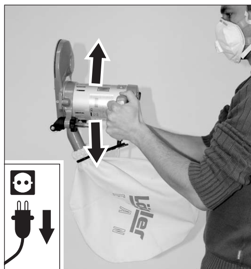
Fig. 30 Before emptying, shake the dust residue into the dust bag.
