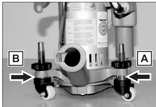
Fig. 68 The sanding zone of the machine is too much to the left means, the right guide roller ( A ) is lifting the machine more than the left guide roller ( B ).
