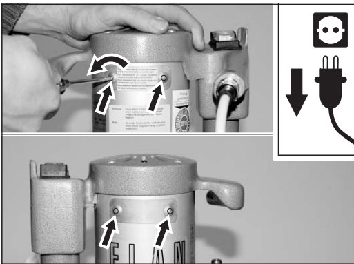
Fig. 50 Unscrew the two covers on the casing tube.
