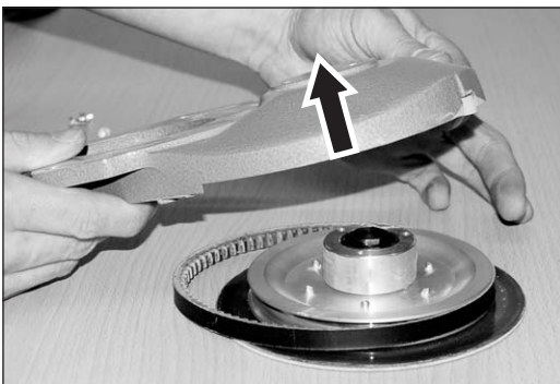
Fig. 39 Remove the attachment from the complete sanding plate.
