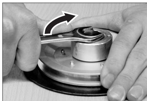
Fig. 43 Unscrew the axle clockwise (left-hand thread) .
