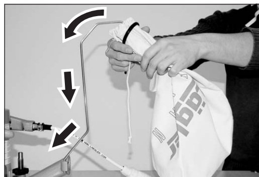
Fig. 6 Place the dust bag over the clamp.
