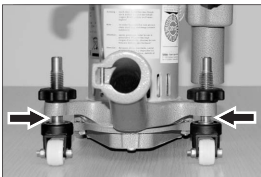
Fig. 59 Steep machine setting for rough sanding tasks.
