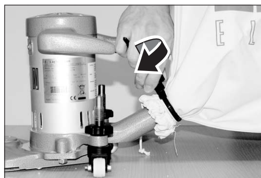
Fig. 8 Sealing the dust bag with the MultiClip.
