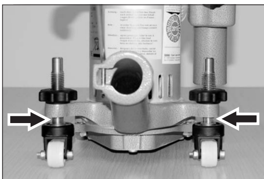
Fig. 59 Steep machine setting for rough sanding tasks.
