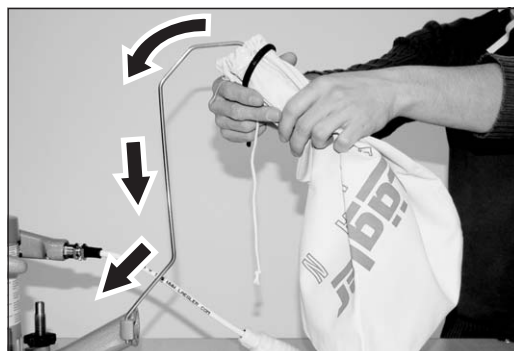
Fig. 6 Place the dust bag over the clamp.
