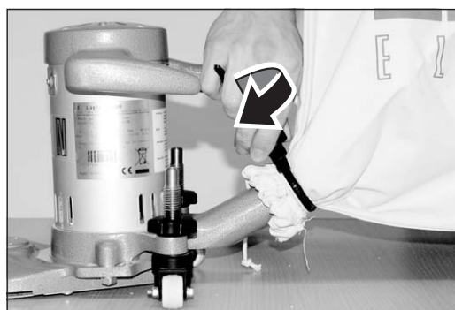
Fig. 8 Sealing the dust bag with the MultiClip.
