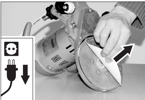
Fig. 21 After removing the sanding disc pull off the Velcro negative and clean the sanding plate.
