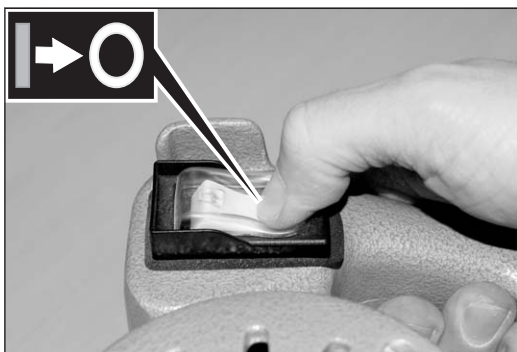
Fig. 12 Push the switch to "O" and the motor will be switched off.
