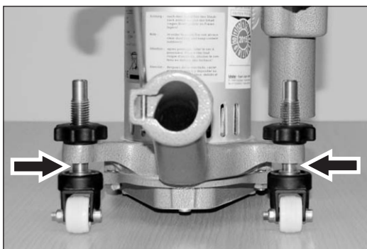
Fig. 56 Setting of the guide rollers for long attachment.
