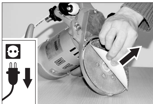
Fig. 16 Simply pull off the Velcro sanding disc.
