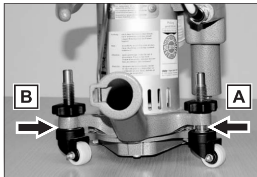
Fig. 68 The sanding zone of the machine is too much to the left means, the right guide roller (A) is lifting the machine more than the left guide roller (B).
