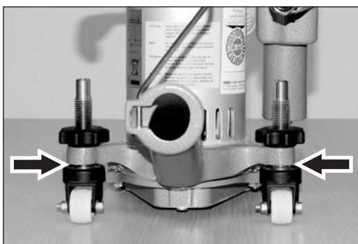
Fig. 57 Flat machine setting for fine sanding tasks.
