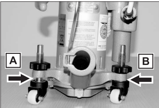
Fig. 66 The sanding zone of the machine is too much to the right means, the left guide roller (A) is lifting the machine more than the right guide roller (B).
