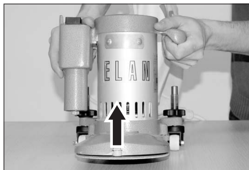
Fig. 10 Always tip the machine backwards slightly before starting or switching off the machine.
